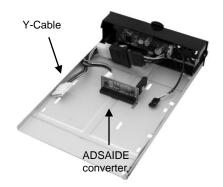
Using the SATA to IDE converter, you can use IDE hard drives on the Zebra enclosure
